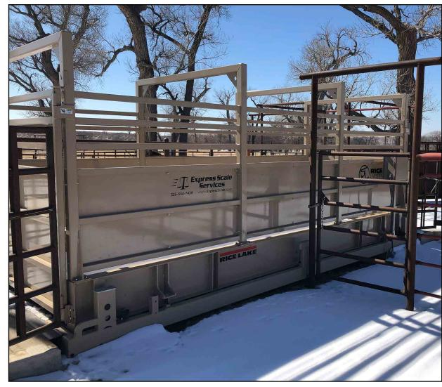
mize the risk of animal injury. It is not uncommon for cattle to slip on dirty platforms when they are being weighed, which is why Rice Lake's livestock scales use recycled plastic and rubber material in a tread-optimized pattern (X-Lug or X-Plank) to provide superior traction. Along with improved animal safety, this will outlast the original scale at this leased ranch property."
